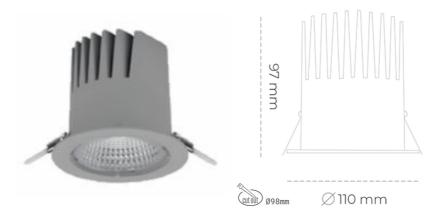
COB 2500 [K] BREAD Light colour CRI Led chip flux 1674 [lm] Luminous flux 1506 [lm] System power 14 [W] Luminaire Efficiency 108 [lm/W] Beam angle 45° Controller ON/OFF
