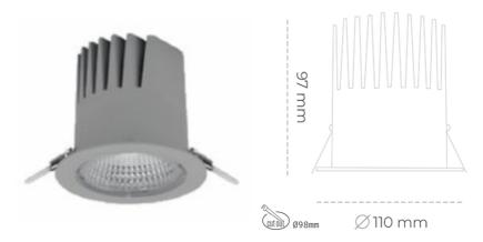
COB 2500 [K] BREAD Light colour CRI 2808 [lm] Led chip flux Luminous flux 2527 [lm] System power 23 [W] Luminaire Efficiency 110 [lm/W] Beam angle 23° Controller ON/OFF MacAdam 3 SDCM
