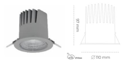
COB 2500 [K] BREAD Light colour CRI Led chip flux 1674 [lm] Luminous flux 1506 [lm] System power 14 [W] Luminaire Efficiency 108 [lm/W] Beam angle 15° Controller ON/OFF MacAdam 3 SDCM
