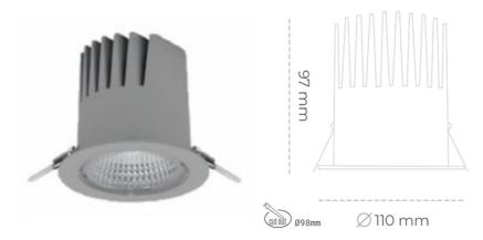
COB 2000 [K] MEAT PINK Light colour CRI Led chip flux 2181 [lm] Luminous flux 1962 [lm] System power 25 [W] Luminaire Efficiency 78 [lm/W] Beam angle 45° Controller ON/OFF MacAdam 3 SDCM
