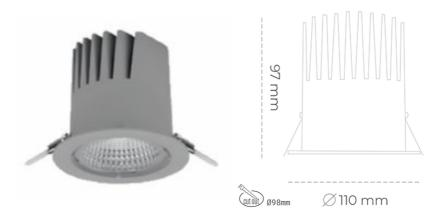
COB 2000 [K] MEAT PINK Light colour CRI 2349 [lm] Led chip flux Luminous flux 2114 [lm] System power 27 [W] Luminaire Efficiency 78 [lm/W] Beam angle 38° Controller ON/OFF MacAdam 3 SDCM
