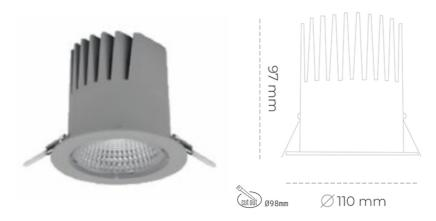
COB 2000 [K] MEAT PINK Light colour CRI Led chip flux 895 [lm] Luminous flux 805 [lm] System power 10 [W] Luminaire Efficiency 81 [lm/W] Beam angle 23° Controller ON/OFF MacAdam 3 SDCM
