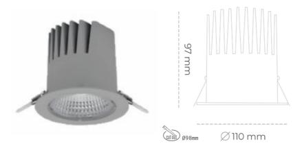
COB 2000 [K] MEAT PINK Light colour CRI Led chip flux 1741 [lm] Luminous flux 1566 [lm] System power 19 [W] Luminaire Efficiency 82 [lm/W] Beam angle 15° Controller ON/OFF MacAdam 3 SDCM
