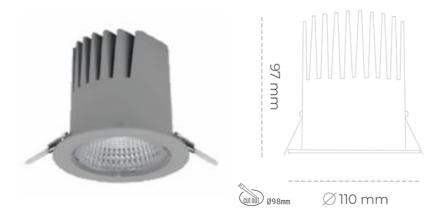
COB Light colour 2700 [K] | CRI Led chip flux 2963 [lm] Luminous flux 2666 [lm] System power 21 [W] Luminaire Efficiency 127 [lm/W] Beam angle 45° Controller ON/OFF MacAdam 3 SDCM
