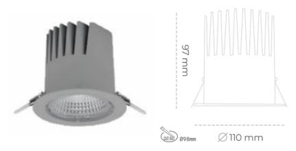
COB 3000 [K] PREMIUM COLOR Light colour CRI 90 Led chip flux 1583 [lm] Luminous flux 1424 [lm] System power 14 [W] Luminaire Efficiency 102 [lm/W] Beam angle 45° Controller ON/OFF MacAdam 3 SDCM
