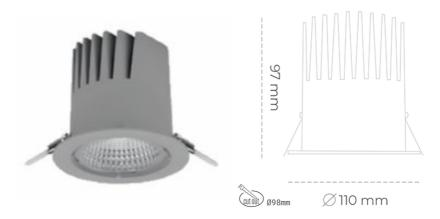
COB 3000 [K] CRI97 Light colour CRI Led chip flux 2601 [lm] Luminous flux 2340 [lm] System power 23 [W] Luminaire Efficiency 102 [lm/W] Beam angle 60° Controller ON/OFF MacAdam 3 SDCM
