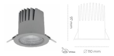
COB 3000 [K] CRI97 Light colour CRI Led chip flux 2990 [lm] Luminous flux 2691 [lm] System power 27 [W] Luminaire Efficiency 100 [lm/W] Beam angle 60° Controller ON/OFF MacAdam 3 SDCM
