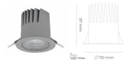
COB 3000 [K] CRI97 Light colour CRI Led chip flux 1575 [lm] Luminous flux 1417 [lm] System power 14 [W] Luminaire Efficiency 101 [lm/W] Beam angle 60° Controller ON/OFF MacAdam 3 SDCM
