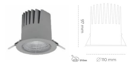
COB 3000 [K] PREMIUM WHITE Light colour CRI 90 Led chip flux 1497 [lm] Luminous flux 1347 [lm] System power 11 [W] Luminaire Efficiency 122 [lm/W] Beam angle 38° Controller ON/OFF MacAdam
