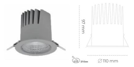
COB 5700 [K] SPECIAL Light colour CRI Led chip flux 2551 [lm] Luminous flux 2295 [lm] System power 19 [W] Luminaire Efficiency 121 [lm/W] Beam angle 60° Controller ON/OFF
