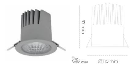
COB 5700 [K] SPECIAL Light colour CRI Led chip flux 1318 [lm] Luminous flux 1186 [lm] System power 10 [W] Luminaire Efficiency 119 [lm/W] Beam angle 45° Controller ON/OFF
