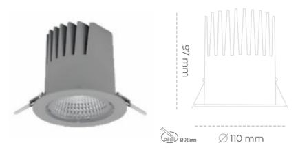
COB 5700 [K] SPECIAL Light colour CRI Led chip flux 3023 [lm] Luminous flux 2720 [lm] System power 23 [W] Luminaire Efficiency 118 [lm/W] Beam angle 15° Controller ON/OFF MacAdam 3 SDCM
