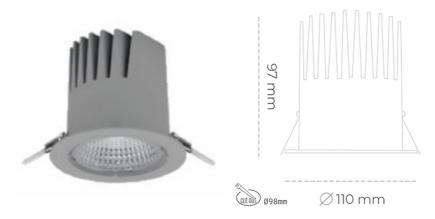
COB 4200 [K] MEAT WHITE Light colour CRI 90 Led chip flux 1023 [lm] Luminous flux 920 [lm] System power 10 [W] Luminaire Efficiency 92 [lm/W] Beam angle 38° Controller ON/OFF MacAdam 3 SDCM
