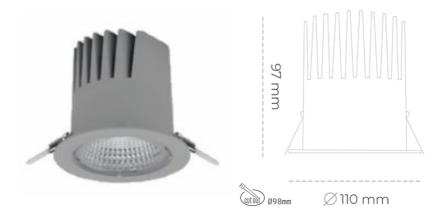
COB 4200 [K] MEAT WHITE Light colour CRI 90 Led chip flux 2159 [lm] Luminous flux 1943 [lm] System power 21 [W] Luminaire Efficiency 93 [lm/W] Beam angle 23° Controller ON/OFF MacAdam 3 SDCM
