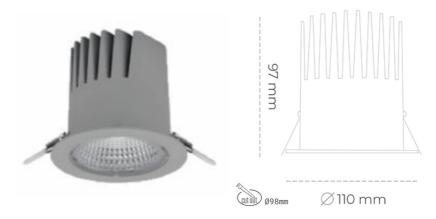
COB 4000 [K] HI EFFICIENT Light colour CRI 90 Led chip flux 2260 [lm] Luminous flux 2034 [lm] System power 14 [W] Luminaire Efficiency 145 [lm/W] Beam angle 38° Controller ON/OFF MacAdam 3 SDCM
