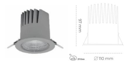
COB 4000 [K] HI EFFICIENT Light colour CRI 90 Led chip flux 3492 [lm] Luminous flux 3142 [lm] System power 21 [W] Luminaire Efficiency 150 [lm/W] Beam angle 23° Controller ON/OFF MacAdam 3 SDCM
