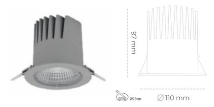
COB 3500 [K] HI EFFICIENT Light colour CRI 90 Led chip flux 4181 [lm] Luminous flux 3762 [lm] System power 27 [W] Luminaire Efficiency 139 [lm/W] Beam angle 38° Controller ON/OFF MacAdam 3 SDCM
