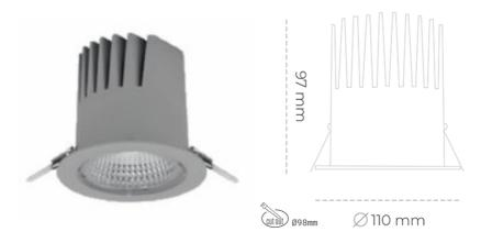
COB 3000 [K] HI EFFICIENT Light colour CRI 90 Led chip flux 3787 [lm] Luminous flux 3408 [lm] System power 23 [W] Luminaire Efficiency 148 [lm/W] Beam angle 38° Controller ON/OFF MacAdam 3 SDCM
