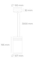
COB Light colour 4000 [K] | CRI 3866 [lm] Led chip flux Luminous flux 3479 [lm] System power 31 [W] Luminaire Efficiency 112 [lm/W] Beam angle 45° Controller ON/OFF MacAdam 3 SDCM
