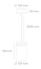
COB Light colour 4000 [K] | CRI 3383 [lm] Led chip flux Luminous flux 3044 [lm] System power 27 [W] Luminaire Efficiency 113 [lm/W] Beam angle 45° Controller ON/OFF MacAdam 3 SDCM
