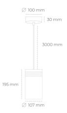
COB Light colour 3000 [K] | CRI Led chip flux 2767 [lm] Luminous flux 2490 [lm] System power 23 [W] Luminaire Efficiency 108 [lm/W] Beam angle 15° Controller ON/OFF MacAdam 3 SDCM
