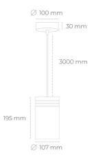
COB Light colour 5000 [K] | CRI Led chip flux 3764 [lm] Luminous flux 3387 [lm] System power 25 [W] Luminaire Efficiency 135 [lm/W] Beam angle 38° Controller ON/OFF MacAdam 3 SDCM
