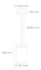
COB Light colour 4000 [K] | CRI 3690 [lm] Led chip flux Luminous flux 3321 [lm] System power 25 [W] Luminaire Efficiency 133 [lm/W] Beam angle 23° Controller ON/OFF MacAdam 3 SDCM
