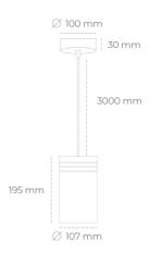
COB Light colour 3500 [K] | CRI 3061 [lm] Led chip flux Luminous flux 2754 [lm] System power 21 [W] Luminaire Efficiency 131 [lm/W] Beam angle 60° Controller ON/OFF MacAdam 3 SDCM
