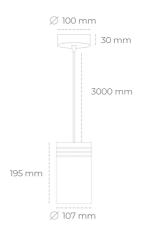
COB Light colour 2700 [K] | CRI Led chip flux 3233 [lm] Luminous flux 2909 [lm] System power 23 [W] Luminaire Efficiency 126 [lm/W] Beam angle 45° Controller ON/OFF MacAdam 3 SDCM
