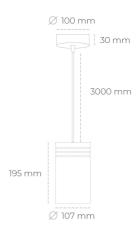
COB 4200 [K] MEAT WHITE Light colour CRI 90 Led chip flux 2159 [lm] Luminous flux 1943 [lm] System power 21 [W] Luminaire Efficiency 93 [lm/W] Beam angle 45° Controller ON/OFF MacAdam 3 SDCM
