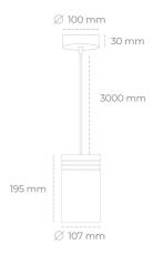
COB 4200 [K] MEAT WHITE Light colour CRI 90 Led chip flux Luminous flux 920 [lm] System power 10 [W] Luminaire Efficiency 92 [lm/W] Beam angle 45° Controller ON/OFF MacAdam 3 SDCM
