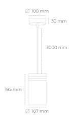
COB 4200 [K] MEAT WHITE Light colour CRI 90 Led chip flux 1412 [lm] Luminous flux 1270 [lm] System power 14 [W] Luminaire Efficiency 91 [lm/W] Beam angle 38° Controller ON/OFF MacAdam 3 SDCM
