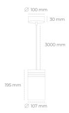
COB 4000 [K] HI EFFICIENT Light colour CRI 90 Led chip flux 4090 [lm] Luminous flux 3681 [lm] System power 25 [W] Luminaire Efficiency 147 [lm/W] Beam angle 60° Controller ON/OFF MacAdam 3 SDCM
