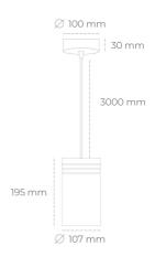
COB 4000 [K] HI EFFICIENT Light colour CRI 90 Led chip flux 3492 [lm] Luminous flux 3142 [lm] System power 21 [W] Luminaire Efficiency 150 [lm/W] Beam angle 60° Controller ON/OFF MacAdam 3 SDCM
