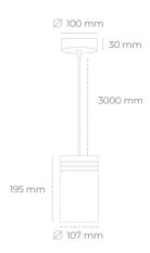
COB 3500 [K] HI EFFICIENT Light colour CRI 90 Led chip flux 4723 [lm] Luminous flux 4250 [lm] System power 31 [W] Luminaire Efficiency 137 [lm/W] Beam angle 45° Controller ON/OFF MacAdam 3 SDCM
