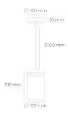
COB 3000 [K] HI EFFICIENT Light colour CRI 90 Led chip flux 4956 [lm] Luminous flux 4460 [lm] System power 31 [W] Luminaire Efficiency 144 [lm/W] Beam angle 38° Controller ON/OFF MacAdam 3 SDCM
