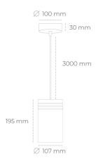
COB Light colour 4000 [K] | CRI Led chip flux 1691 [lm] Luminous flux 1521 [lm] System power 14 [W] Luminaire Efficiency 109 [lm/W] Beam angle 60° Controller ON/OFF MacAdam 3 SDCM
