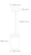
COB Light colour 4000 [K] | CRI 3866 [lm] Led chip flux Luminous flux 3479 [lm] System power 31 [W] Luminaire Efficiency 112 [lm/W] Beam angle 38° Controller ON/OFF MacAdam 3 SDCM
