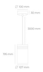
COB Light colour 4000 [K] | CRI Led chip flux 1691 [lm] Luminous flux 1521 [lm] System power 14 [W] Luminaire Efficiency 109 [lm/W] Beam angle 15° Controller ON/OFF MacAdam 3 SDCM
