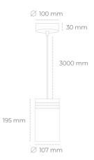
COB Light colour 3000 [K] | CRI Led chip flux 3227 [lm] Luminous flux 2904 [lm] System power 27 [W] Luminaire Efficiency 108 [lm/W] Beam angle 15° Controller ON/OFF MacAdam 3 SDCM
