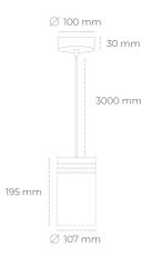
COB Light colour 3000 [K] | CRI Led chip flux 2767 [lm] Luminous flux 2490 [lm] System power 23 [W] Luminaire Efficiency 108 [lm/W] Beam angle 15° Controller ON/OFF MacAdam 3 SDCM
