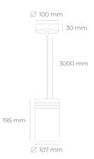
COB Light colour 2700 [K] | CRI Led chip flux 2667 [lm] Luminous flux 2400 [lm] System power 23 [W] Luminaire Efficiency 104 [lm/W] Beam angle 45° Controller ON/OFF MacAdam 3 SDCM
