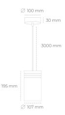
COB Light colour 2700 [K] | CRI Led chip flux 1111 [lm] Luminous flux 999 [lm] System power 10 [W] Luminaire Efficiency 100 [lm/W] Beam angle 38° Controller ON/OFF MacAdam 3 SDCM
