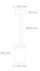
COB Light colour 5000 [K] | CRI Led chip flux 3185 [lm] Luminous flux 2866 [lm] System power 21 [W] Luminaire Efficiency 136 [lm/W] Beam angle 38° Controller ON/OFF MacAdam 3 SDCM
