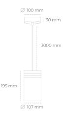
COB Light colour 5000 [K] | CRI Led chip flux 1447 [lm] Luminous flux 1302 [lm] System power 10 [W] Luminaire Efficiency 130 [lm/W] Beam angle 38° Controller ON/OFF MacAdam 3 SDCM
