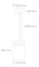
COB Light colour 4000 [K] | CRI Led chip flux 3122 [lm] Luminous flux 2809 [lm] System power 21 [W] Luminaire Efficiency 134 [lm/W] Beam angle 38° Controller ON/OFF MacAdam 3 SDCM
