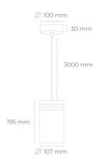
COB Light colour 3500 [K] | CRI Led chip flux 1391 [lm] Luminous flux 1251 [lm] System power 10 [W] Luminaire Efficiency 125 [lm/W] Beam angle 60° Controller ON/OFF MacAdam 3 SDCM
