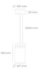
COB Light colour 3500 [K] | CRI 3340 [lm] Led chip flux Luminous flux 3006 [lm] System power 23 [W] Luminaire Efficiency 131 [lm/W] Beam angle 38° Controller ON/OFF MacAdam 3 SDCM
