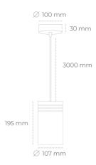
COB Light colour 3000 [K] | CRI Led chip flux 3811 [lm] Luminous flux 3429 [lm] System power 27 [W] Luminaire Efficiency 127 [lm/W] Beam angle 45° Controller ON/OFF MacAdam 3 SDCM
