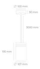
COB Light colour 2700 [K] | CRI Led chip flux 1886 [lm] Luminous flux 1697 [lm] System power 13 [W] Luminaire Efficiency 131 [lm/W] Beam angle 38° Controller ON/OFF MacAdam 3 SDCM
